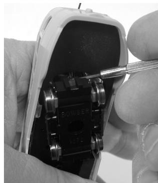
**2.** Start with the rear end. With body spread from step 1, slide a small screwdriver into the truck opening and pull the mechanism out a little. Repeat step 1 and 2 for front end.
