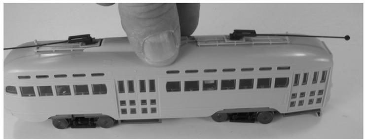
**7.** Reassemble the circuit board to the frame. Be sure the wires do not touch the flywheel or the universal shaft. Place the mechanism on your table. Align the body and press the body onto the frame. The window hooks will engage the frame.
