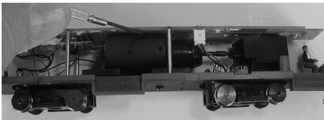
**3.** Gently pry circuit board off the mounting posts.
