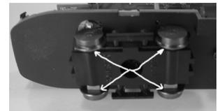
**6.** Oil all 8 axles where it pass through the bearing or pickup (brass plate) One drop is enough.
