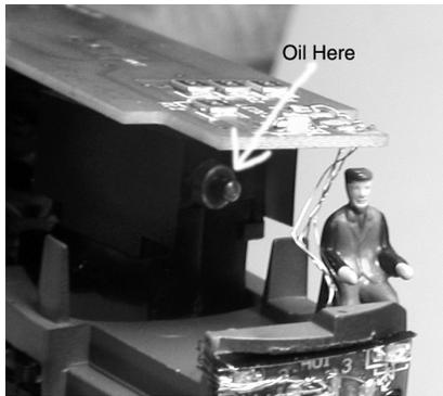
**5.** Oil both ends of worm shaft (shown) where it passes thru the bearing. Bearing is behind the driver figure in the photo. Also oil other end of shaft.
