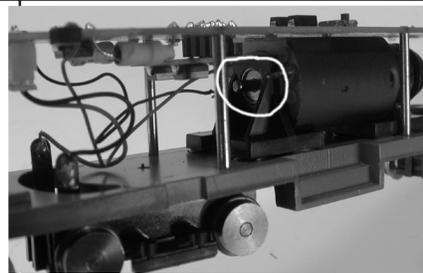
**4.** Oil both ends of motor shaft where it passes thru the motor bearing. The flywheel end requires a thin tube oiler to get between the flywheel and the motor housing.
